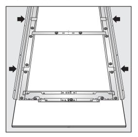
■ Insert the angle trim <sup>③</sup> as far as it will go in the spaces provided in the mounting frame.
